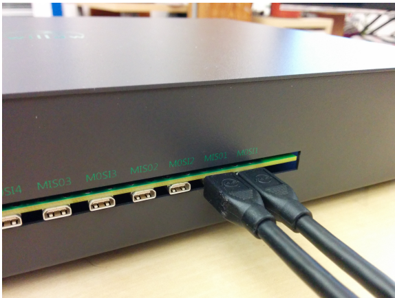
Figure 3. - Example of Datanode paired-ports MISO1 and MOSI1 connected to a Headstage's MISO/MOSI ports
